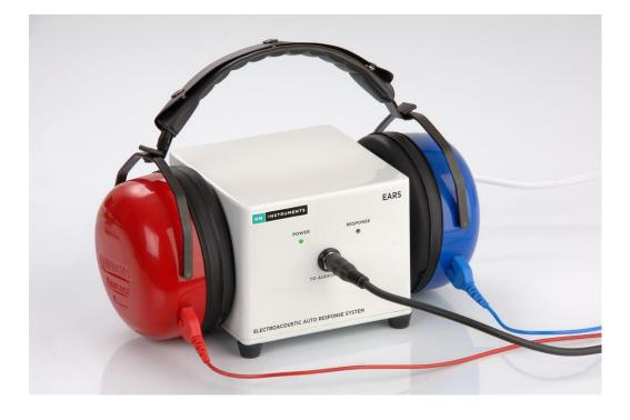
Ensure the headphones are the correct pair for the audiometer being tested
