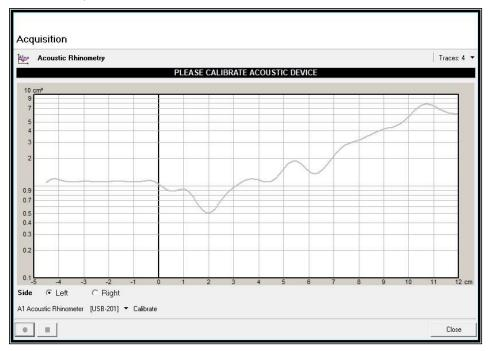
2) If a calibration file is found, you will see the screen below and can proceed to testing, or alternatively you can refresh the calibration by ensuring the A1 is switched on and that the calibration plug is correctly fitted, and clicking on the button marked **Calibrate**.
