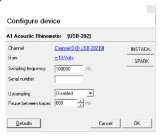
When the USB interface is installed **(USB-202)**, the window will show: the board number [0], the channel used for the microphone (which, by default, is channel 0), the selected gain setting (±10 Volts), the basic sampling frequency (100kHz), the upsampling option will be disabled, and the pause between each measurement (700 mS). These are the default settings for a USB-202 interface and should not normally be changed.
