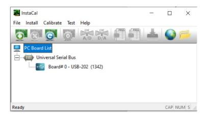
When InstaCal shows the screen above, (shown for a 202 module) USB installation is complete and InstaCal can be closed.
