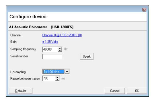
When you click on **Calibrate** in the test acquisition window, you should have the A1 powered up, with the calibration plug fully inserted into the A1 sound tube. An updated calibration file will be generated and saved to the default folder – the same directory to which the program was installed.
