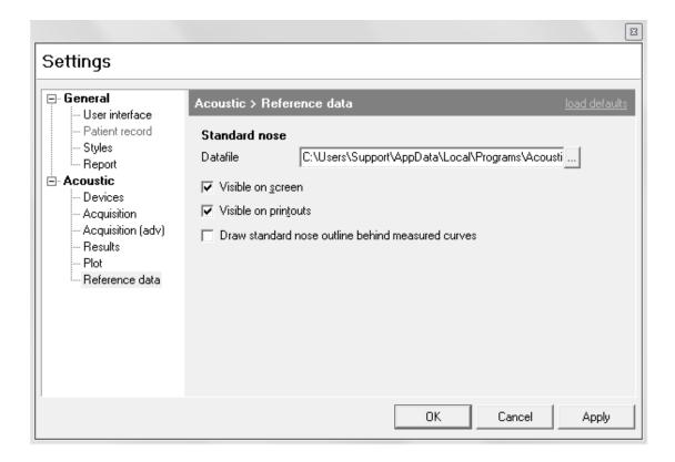
Validation of system performance can be made by comparing a theoretical **Standard nose** curve, with that obtained when making a measurement on a **Standard nose** model.
